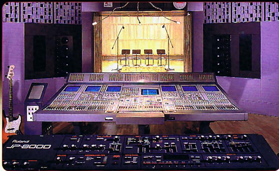
A view from the master control room looks on to the XM Live Performance Studio where the 48-track Sony Oxford digital console allows engineers to record, mix and re-master performers' sound.
