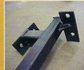
THE HYDRAULIC PUNCH & SHEAR (RIGHT) IS USED TO FABRICATE CUSTOM BRACKETS (ABOVE). AI EVEN SUPPLIES THESE TO OTHER SHOPS
