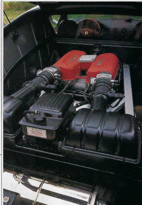
LORD OF THE HIGHWAYS: Sometimes, Kramer prefers to listen to the Ferrari's 400-horsepower, all-aluminum V8 engine. Can you really blame him?
