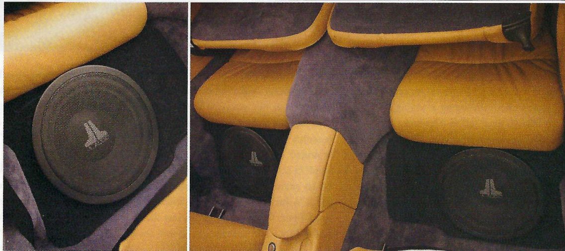
PANDORA'S SUB BOX: Two JL Audio 10-inch subwoofers are tucked below the Porsche's back seat (far right); each sub, running free-air, is mounted in a baffle that tapers from the top of the back seat to the rear floorboard (right).
