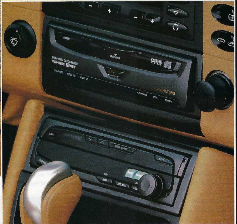
GET IT UP: The Alpine multimedia head unit was installed in a stock storage pocket below the dash (above right) so its 6.5-inch color monitor (above) wouldn't block the climate controls; an Alpine DVD player fit in the stock-radio location above it (right).
