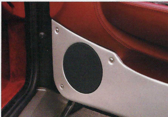
NO SURPRISE: Speakers from a JL Audio component set dropped into the stock locales—the mid in the bottom of each door (above), the tweet in each sail panel (left).
