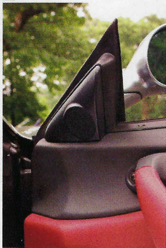
NO SURPRISE: Speakers from a JL Audio component set dropped into the stock locales—the mid in the bottom of each door (above), the tweet in each sail panel (left).
