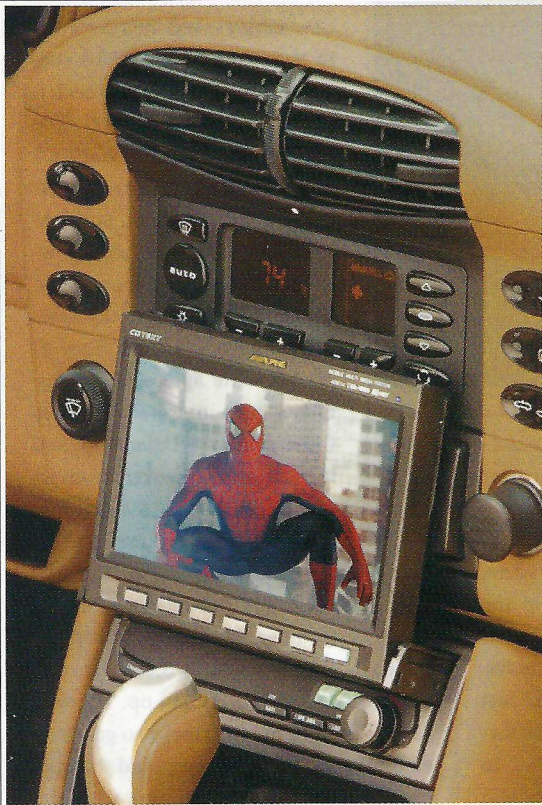
GET IT UP: The Alpine multimedia head unit was installed in a stock storage pocket below the dash (above right) so its 6.5-inch color monitor (above) wouldn't block the climate controls; an Alpine DVD player fit in the stock-radio location above it (right).
