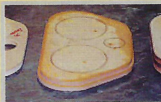
A wooden top and bottom jig surround a Bond-O ring built using Fukuda's "technique"
