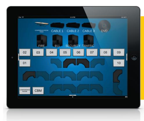
The team at AVS Systems created a customized user interface replicating the seating position of each operator on an iPad Mini.
