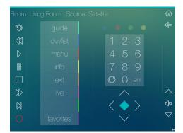
This screen shows control of the satellite receiver in the living room. Each vertical array of control commands are called drawers. Notice that the drawer on the far right for controlling HOME, BACK, VOLUME AND MUTE remain present even as the user changes screens. This gives the user constant access to critical functions across all panels (screens).
