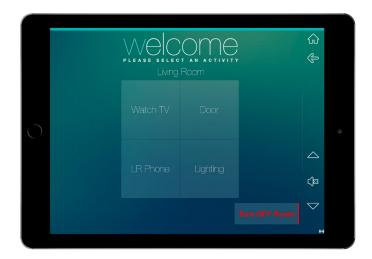
This screen shows the view once the user has selected the Living Room. Within the cluster of four large buttons, the "door" button enables the user to activate an automated door opener/closer. This gives the user much desired security and privacy controlled from the iPad.
