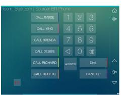
This screen gives the user control of the bedroom landline telephone neatly equipped with "PRESET" buttons for frequently called numbers, "ANSWER," "DIAL" and "HANG-UP" buttons. The user can call all handsets (functions as room-to-room intercom) associated with the base phone and trigger a distinctive ring so that the person on the receiving end knows who is calling. This screen also contains a "911" option in case of emergency.
