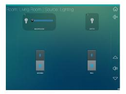
This screen is an example of lighting control for the living room. The user can control lights in the living room as well as other rooms, with some lighting loads being dimmable and some being on/off. The independent switches on the screen can accommodate 2-way or 3-way switching circuits as needed.
