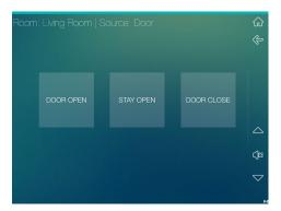
This screen gives the user control of the living room door. The challenge here was to give the user a "STAY OPEN" option so they don't have to rush during ingress or egress from the room. The user is able to "park" the door in the open or closed position as well as rely on standard delay times up to about 45-seconds before the door auto-closes.
