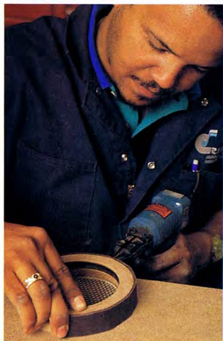
Baffle house: Kevan R. Budrow attaches waterproof panelboard to the outside of the baffle, creating a recessed area for the grille ring to fit into (left); the perfect pair—the grille ring with its steel mesh leans on its soon-to-be companion, the baffle ring (above).
