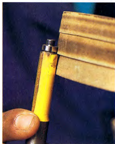
Meet the ringleaders: The grille, the baffle, and the original template rings spend a relaxing moment or two with the router bits and holesaws that created them (above); the flush-trim bit is used to cut the grille 0.125 inch smaller in diameter than the baffle and template rings above it (below).
