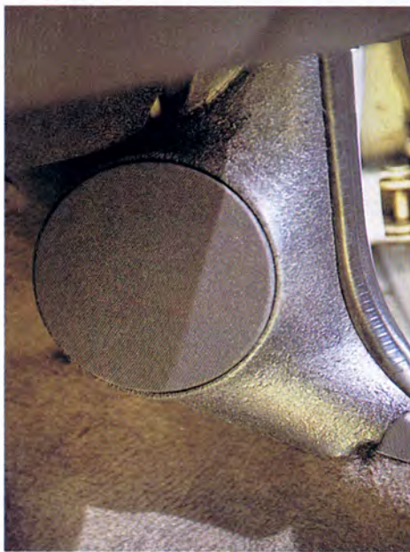
Pod, people: A finished pod in the kickpanel (above) and the original before the install took place (top). Note that the speaker hardly protrudes into the passenger's personal space.
