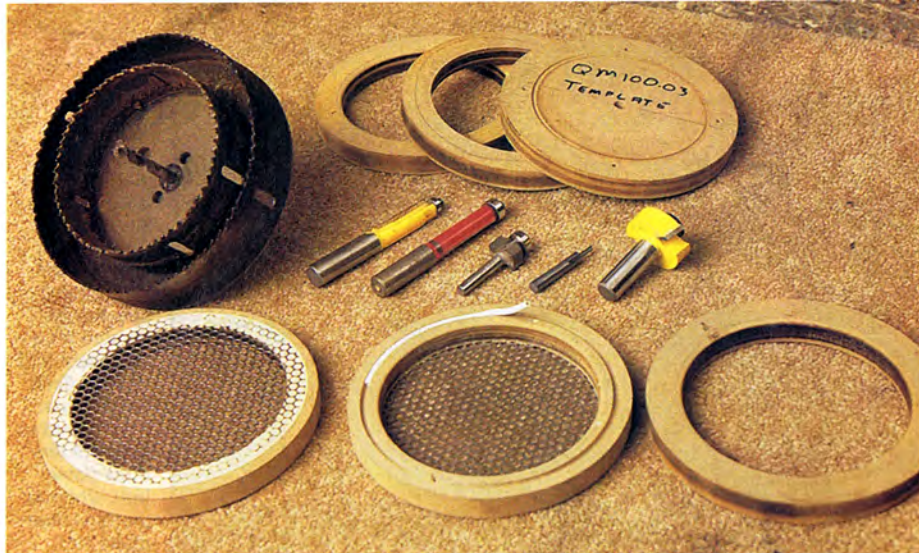
Meet the ringleaders: The grille, the baffle, and the original template rings spend a relaxing moment or two with the router bits and holesaws that created them (above); the flush-trim bit is used to cut the grille 0.125 inch smaller in diameter than the baffle and template rings above it (below).
