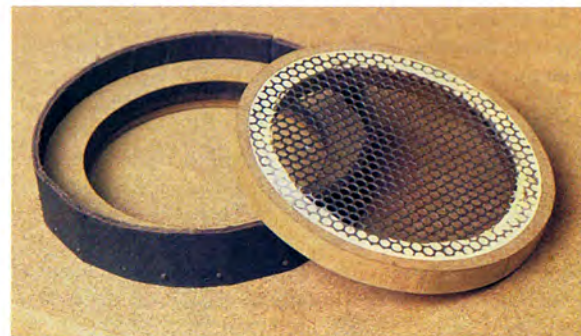
Baffle house: Kevan R. Budrow attaches waterproof panelboard to the outside of the baffle, creating a recessed area for the grille ring to fit into (left); the perfect pair—the grille ring with its steel mesh leans on its soon-to-be companion, the baffle ring (above).
