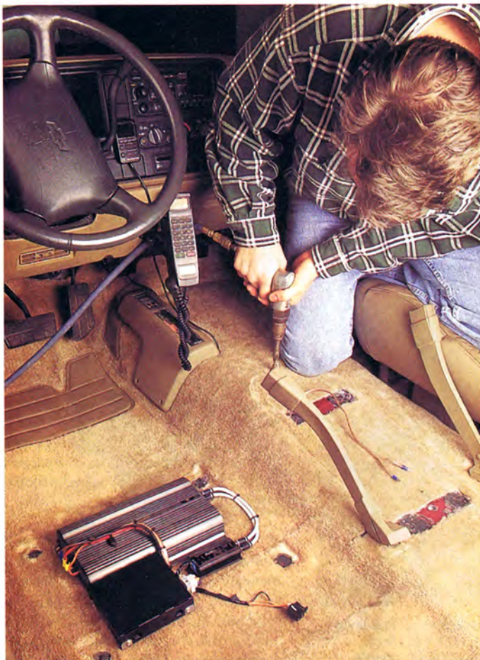
Left: After marking the Suburban's carpet with the soft wax that's provided with the woofer kit, Argo drills two mounting holes through the floor for the finished Stealthbox console. Right: When drilling through the floor pan, keep the drill bit perpendicular to the floor
