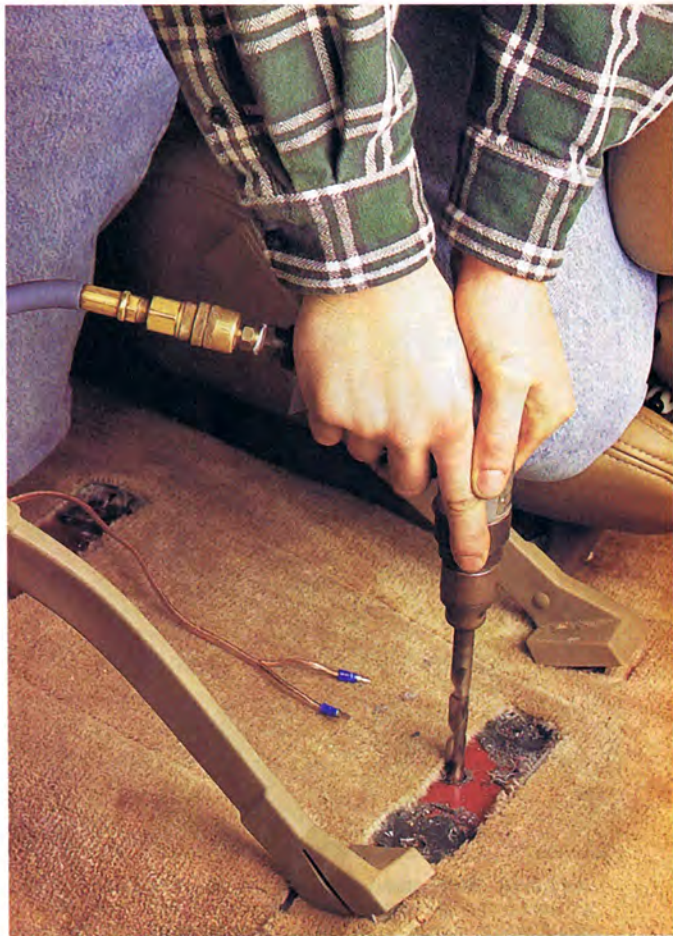
Left: After marking the Suburban's carpet with the soft wax that's provided with the woofer kit, Argo drills two mounting holes through the floor for the finished Stealthbox console. Right: When drilling through the floor pan, keep the drill bit perpendicular to the floor
