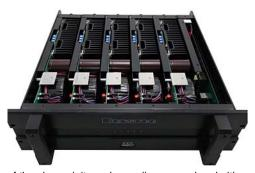
channel is indeed its own amplifier. In fact, should something go wrong with one of the channel, it can be easily removed and either fixed or replaced with another module. One of the company's most impressive features is a 20-year warranty, so you need not worry about service for quite some time.
