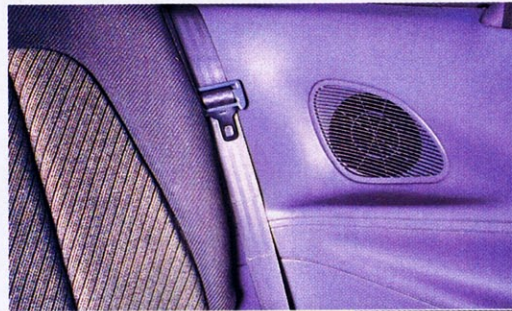
Left: An adaptor was used to fit round speaker in rear side panel's stock oval cut-out.
