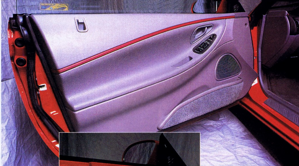
Above: MB Quart speakers fit into the door's stock locations. Right: With door panel removed, damping material is visible.
