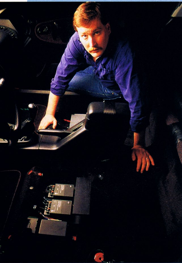
The a/d/s/ amplifiers and crossovers were mounted on the floor beneath the seats.
