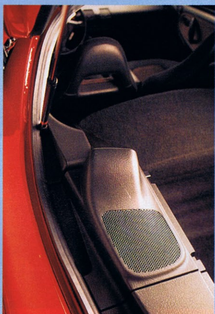
Right: Stock grille in hatch area conceals an a/d/s/ 200i plate speaker.
