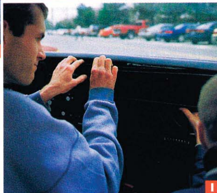
RIPPED OFF: Listening for the Python's clicking light-flash relay, the duo rip out the glove box to find the brain. Don't forget, the car won't start until the alarm is defeated. Taking a cue from the LeBaron install, the boys tear out the radio (G), thinking the brain might be there—but it isn't, so the hunt continues. Klisus and Steiner ditch the tactful approach and simply tear off the dash (H, I). Thieves prefer not to be this destructive if the car is being stolen as a parts donor; however, as more time passes, desperate measures become necessary. With the right side of the dash now destroyed, Klisus accesses the Python brain and unplugs it (J). Finally, 3:20 from the start of the theft attempt, the alarm is disabled. The ignition switch is now vulnerable. An experienced thief would next pop out the GM switch in a few seconds and have the car running, but we left the ignition key for Klisus rather than have him smash the steering column. The difference between using the key and popping the switch is 10 to 15 seconds. So, at 3:25 into the heist, the big, bad Caprice is finally running.
