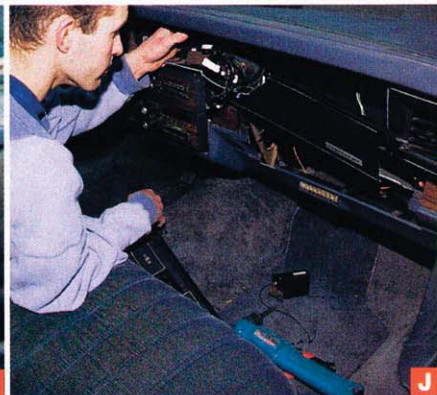
RIPPED OFF: Listening for the Python's clicking light-flash relay, the duo rip out the glove box to find the brain. Don't forget, the car won't start until the alarm is defeated. Taking a cue from the LeBaron install, the boys tear out the radio (G), thinking the brain might be there—but it isn't, so the hunt continues. Klisus and Steiner ditch the tactful approach and simply tear off the dash (H, I). Thieves prefer not to be this destructive if the car is being stolen as a parts donor; however, as more time passes, desperate measures become necessary. With the right side of the dash now destroyed, Klisus accesses the Python brain and unplugs it (J). Finally, 3:20 from the start of the theft attempt, the alarm is disabled. The ignition switch is now vulnerable. An experienced thief would next pop out the GM switch in a few seconds and have the car running, but we left the ignition key for Klisus rather than have him smash the steering column. The difference between using the key and popping the switch is 10 to 15 seconds. So, at 3:25 into the heist, the big, bad Caprice is finally running.
