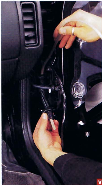
WIRED FOR SOUND: To run speaker wires into the Saturn's front doors, Samudosky used a 4-foot wire tie as a snake (V). Concerned that the stiff wire tie might puncture the rubber boot as he worked it through, Samudosky loosened the boot at each end so that he could gently insert his fingers into the tube and pull the snake through without causing any harm to the tubing (W).
