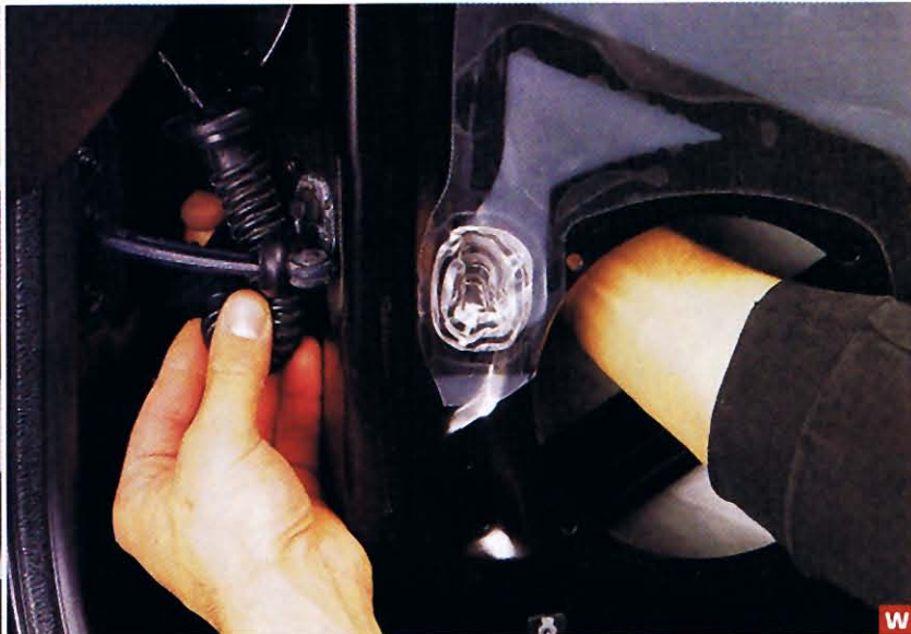
WIRED FOR SOUND: To run speaker wires into the Saturn's front doors, Samudosky used a 4-foot wire tie as a snake (V). Concerned that the stiff wire tie might puncture the rubber boot as he worked it through, Samudosky loosened the boot at each end so that he could gently insert his fingers into the tube and pull the snake through without causing any harm to the tubing (W).
