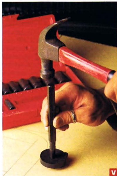
BLANK GENERATION: Using a factory-drilled hole to get through the Saturn's firewall, Samudosky turned an unused rubber plug, known as a blank, into a grommet with a hole punch (V) and ran the power wire through it (W). It's essential to fuse the amplifier's main power lead close to the battery to prevent fire by way of a short circuit (X).
