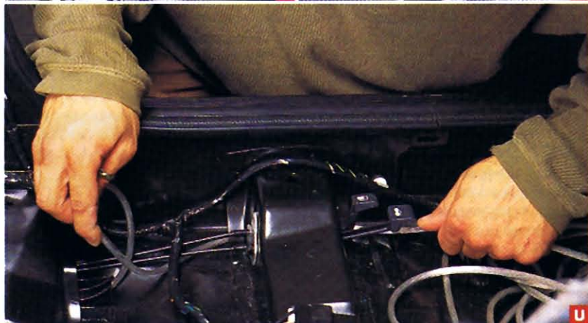
BRUSH JOB: When grounding your amp to the vehicle's chassis, it's important to remove any paint or primer from the area with a stiff wire brush (S). Use a quality ring connector and a self-tapping screw with a star washer to make a solid ground connection (T). Always run the amp's main 12-volt power source up the side of the vehicle that the battery is located on (U).
