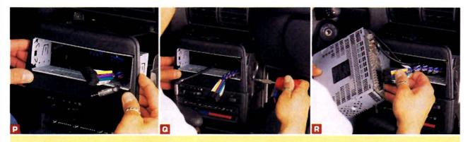
HOME STRETCH: Mount the sleeve/kit assembly (P) and secure it using the supplied screws or via the factory screws whenever possible (Q). When all is snug, plug the wire harness and antenna adaptor into the back of the aftermarket receiver and carefully insert the head into the sleeve/kit assembly (R).
