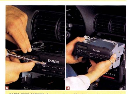
RADIO-FREE SATURN: Once the trim and/or dash panels are removed, it's time to remove the actual radio. (This process will vary from vehicle to vehicle.) With the shroud removed, use a 7-millimeter socket on a ½-inch ratchet with extension (G) to take out the bolts that hold the stock head in place and then carefully free the radio from its mount (H).
