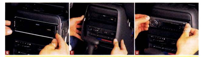
HEAD END: Snap the supplied plastic radio trim ring on the front of the head unit (S), reinstall all of the trim or dash panels (T), and pop on the receiver's faceplate (U). Voilà! You're done (V, below). Nice job!
