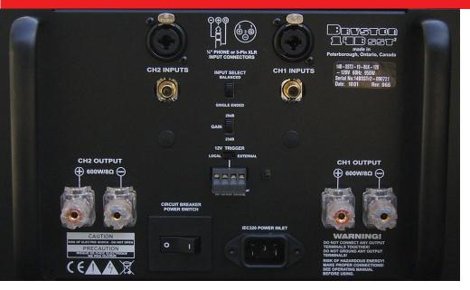
SST2 is rated at 600 watts rms per channel output into 8 ohms. That is only 3 dB less in loudness capability than 1,200 watts (power is an exponential variable).
