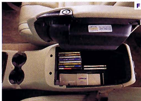
CHANGE THE CHANGER: Audio Coupe replaced the stock 6-disc changer in the center console with a JVC 12-disc model (F).
