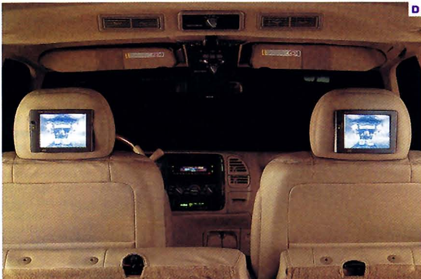
CADDY THEATER: A pair of JVC color LCD monitors are flush-mounted into the backs of the front-seat headrests (D) and attached with Velcro. A JVC VCR shows its stuff from under the passenger's-side rear seat (E).
