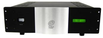
input voltage. Should a fault condition occur (anything lower than 85 or higher than 135 volts), the Torus AVR units can be user-programmed to automatically turn off, protecting all associated electronics. "By adding the AVR series to the existing Torus lineup, we now have compelling products that provide power isolation, automatic voltage regulation, and automatic voltage protection all within a single component," explained sales VP James Tanner.
